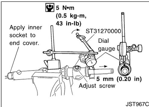
21. Rotate the pinion counterclockwise as far as it will go.
