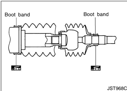
25. Before assembling the boot, temporarily install the boot band to the larger-diameter side.
