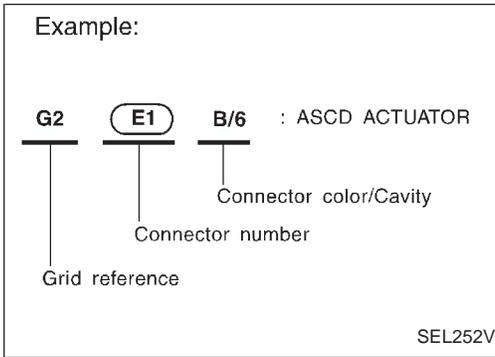
The following Harness Layouts use a map style grid to help locate connectors on the drawings:
