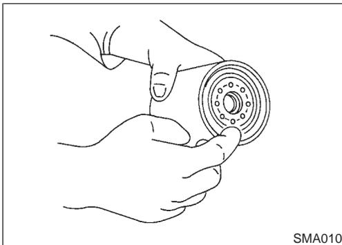
2. Before installing new oil filter, clean the oil filter mounting surface on cylinder block, and coat the rubber seal of oil filter with a little engine oil.
