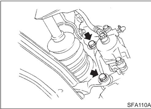
3. Remove brake caliper assembly and rotor.
