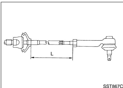
23. Tighten outer socket lock nut.
