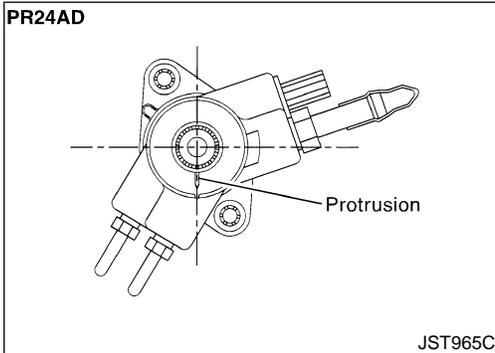
13. Ensure that the rack is centered. Install rear cover cap so that its protrusion is positioned as shown in figure.
