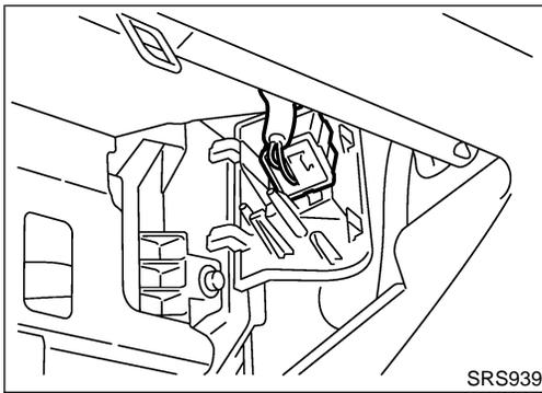
3. Connect air bag module connector to air bag harness connector.
