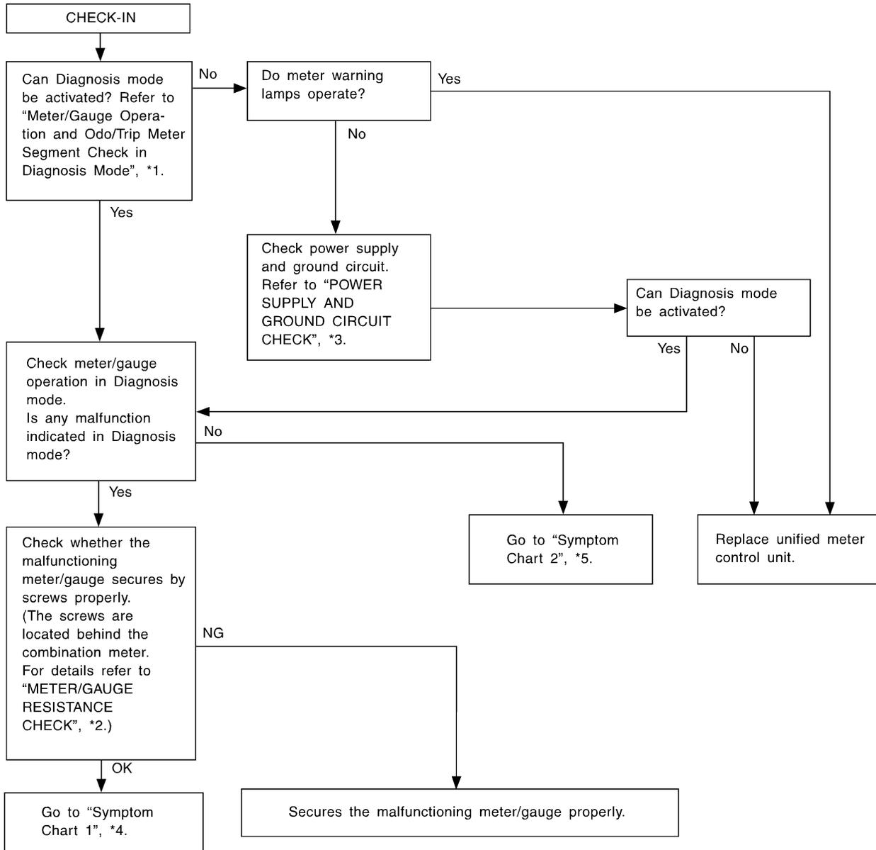
\*1: Meter/Gauge Operation and Odo/Trip Meter Segment Check in Diagnosis Mode (EL-64)
