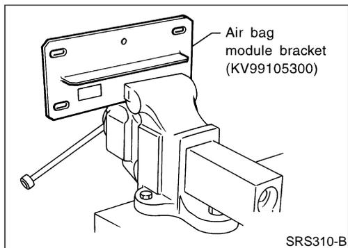
2. Firmly secure air bag module bracket (SST: KV99105300) in a vise.
