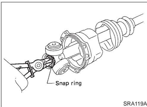
5. Pry off snap ring, then remove spider assembly.
