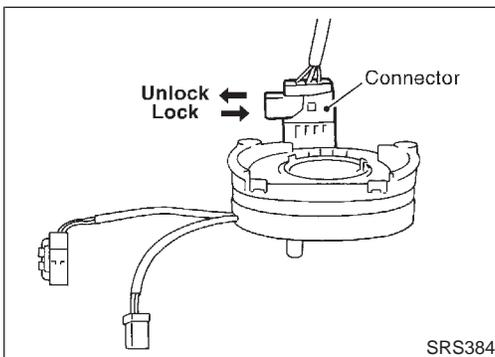
8. Unlock the spiral cable connector. Disconnect connectors and remove the four screws. The spiral cable can then be removed.
