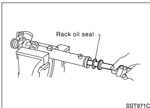
5. Install rack oil seal (Inner) with rack assembly.
