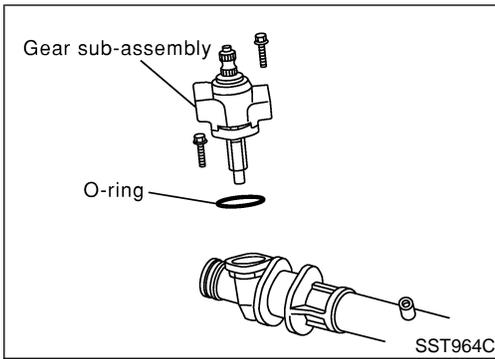
11. Install O-rings to gear sub-assembly.
