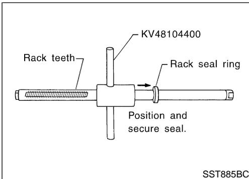
3. Using Tool, compress rack seal ring securely onto rack.
