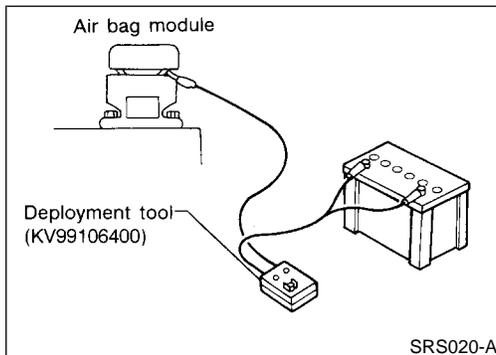
4. Connect deployment tool adapter (SST: KV99108300) to deployment tool (SST: KV99106400) connector and air bag module connector.
