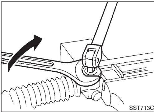
19. Prevent adjusting screw from turning, and tighten lock nut to specified torque.
