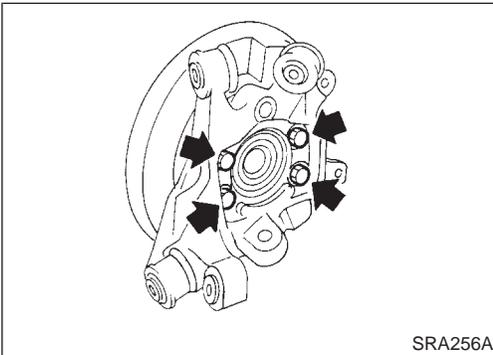
5. Remove wheel bearing with flange, and wheel hub from axle housing.
