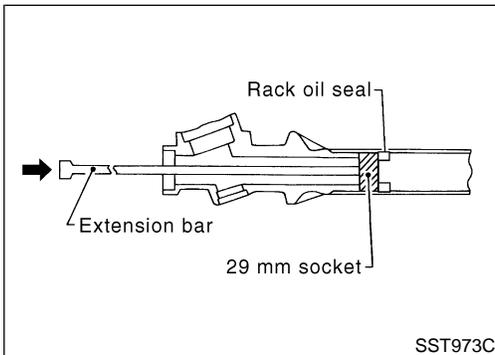
10. Remove rack oil seal (inner) using tape wrapped socket and extension bar.
