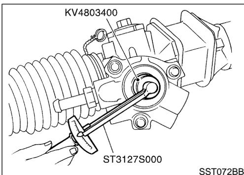
16. Measure pinion rotating torque within the range of 180° from neutral position.
