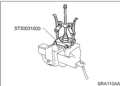
3. Remove inner race from hub using a bearing replacer/puller.
