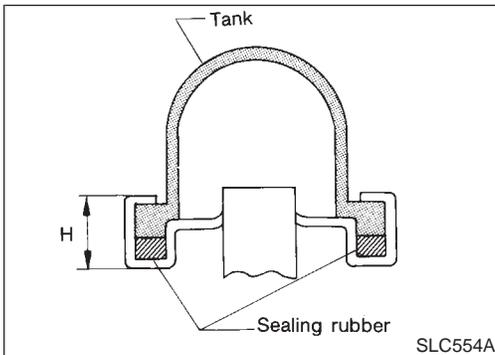
5. Make sure that the rim is completely crimped down.
