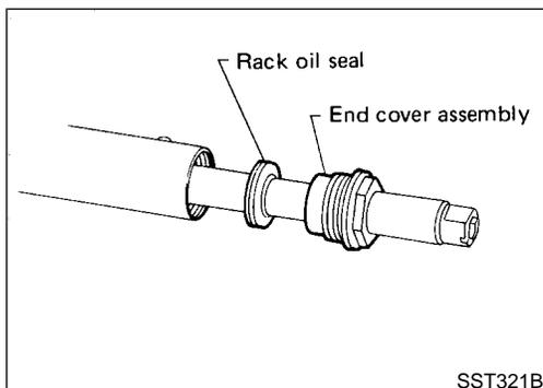
6. Insert rack oil seal (Outer) and end cover assembly to rack. Then install end cover assembly.
