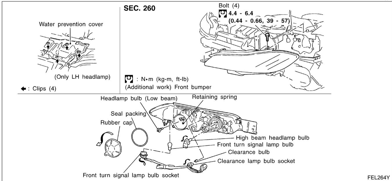
The headlamp is a semi-sealed beam type which uses a replaceable halogen bulb. The bulb can be replaced from the engine compartment side without removing the headlamp body.
