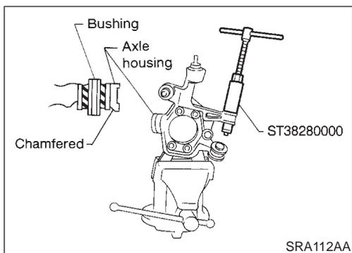
2. Ensure axle housing bore is free from scratches or deformities before pressing bushing into it.
