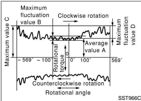
20. Measure the rotational torque of the pinion gear to confirm that it is within the specified torque range. If it is out of the specified range, readjust it. If it is still out of specifications after readjustment, replace the power steering gear.
