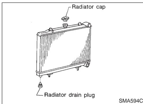
2. Open radiator drain plug at the bottom of radiator and remove radiator cap.
