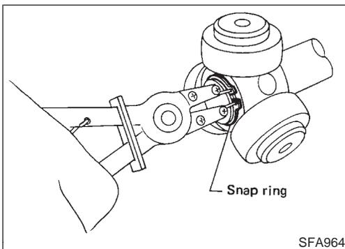
4. Pry off snap ring, then remove spider assembly.
