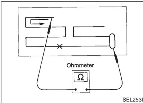
2. To locate broken point, move probe along element. Tester needle will swing abruptly when probe passes the point.
