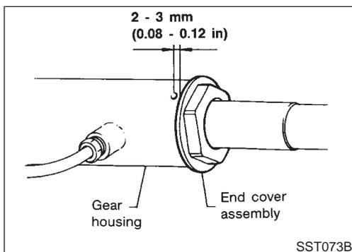
9. Fasten end cover assembly to gear housing by staking.
