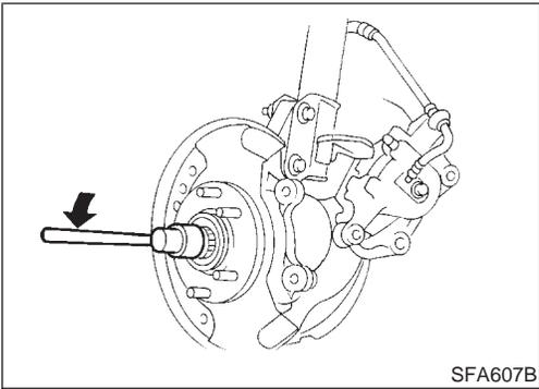
1. Remove wheel bearing lock nut. Remove wheel hub from spindle.
