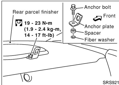
**Replace anchor bolts if they are deformed or worn out.**
