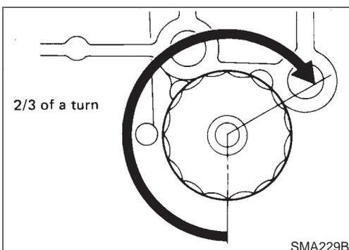
3. Screw in the oil filter until a slight resistance is felt, then tighten additionally more than 2/3 turn.
