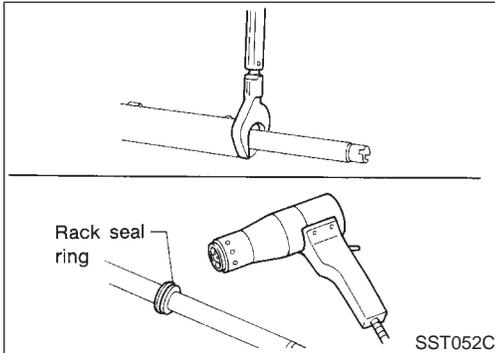
7. Remove end cover assembly with a suitable tool.
